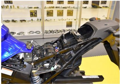
Locate the gear position sensor connector at the left side.
