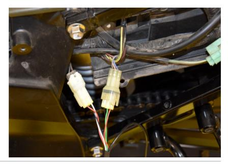
Connect the GPAT G2 Red wire to the Orange/Green wire of the diagnostic 6-pole connector.
